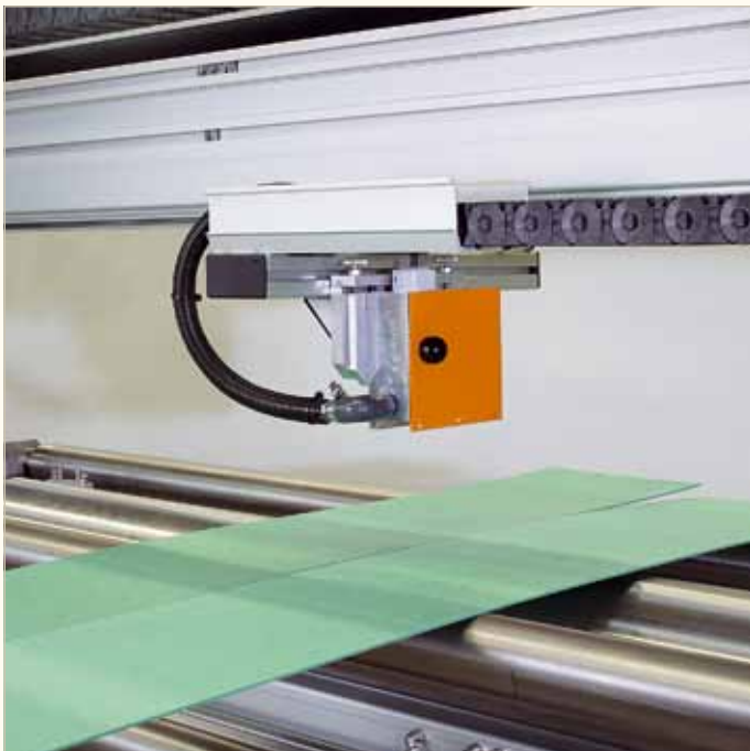
Measurement of impact sound insulation with the DML 5000
