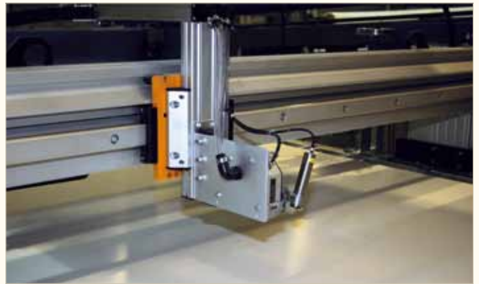
Traversing laser measurement of PVC sheets at Simona
