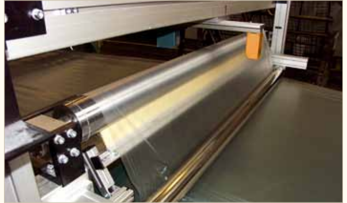
Laser measurement of plastic film at Metzeler
