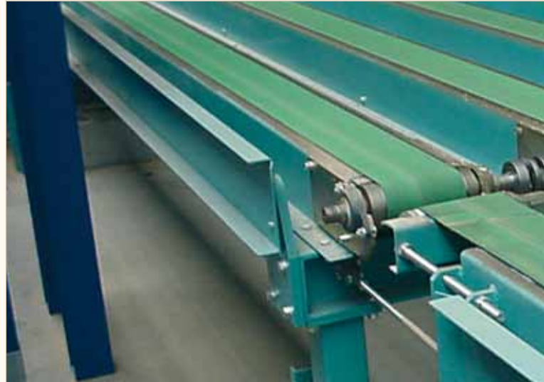
Board scale with belt conveyor
